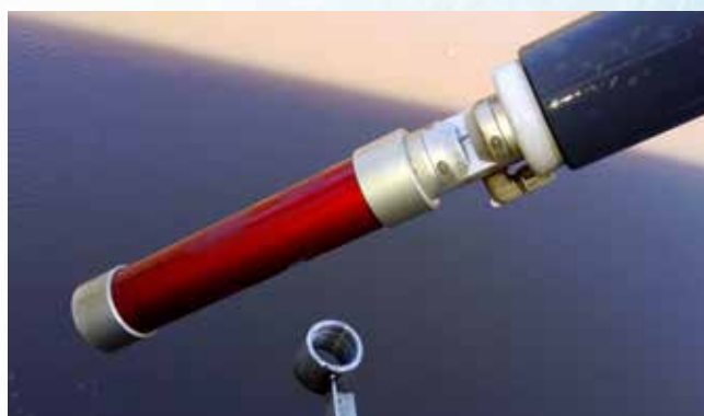
Fig. 38. This device uses automatic compressed air cleaning before each measurement. The figure shows that the hardware itself is dirty, but the optical window is clean (left hand figure). In the figure on the right, the device has been completely cleaned.
