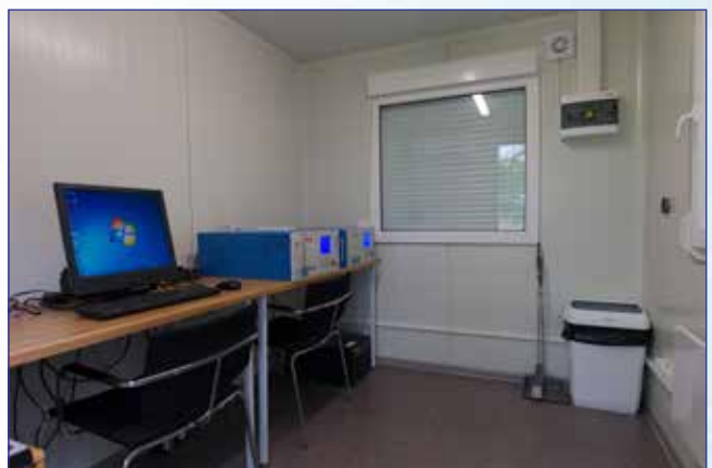
Fig. 23 Indoor view of the new measurement container. On the table from left to right a measurement computer, a sulphur dioxide monitor and an ozone monitor. In the corner under the table is an uninterruptible power supply (UPS).
