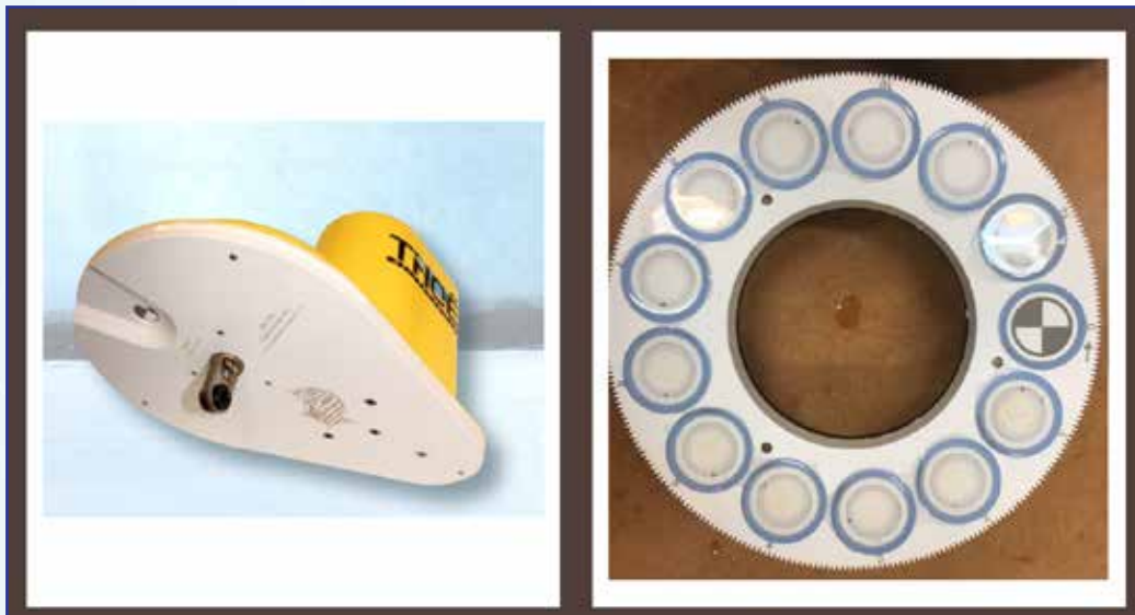
Fig. 16. The PO 4 -P device including the passive collectors (DGT, see also www.dgtresearch.com )
